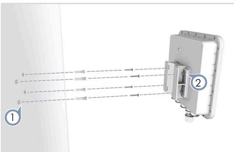
1. At the installation location on the wall, use the mounting bracket to mark four holes for the wall plugs and screws. The bracket must be installed with the marking "UP" at the top.
