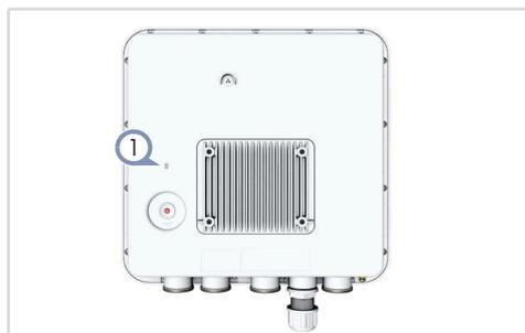
1. When operating normally, the Power/Status LED should be on yellow green. Blinking indicates the device is booting up.
