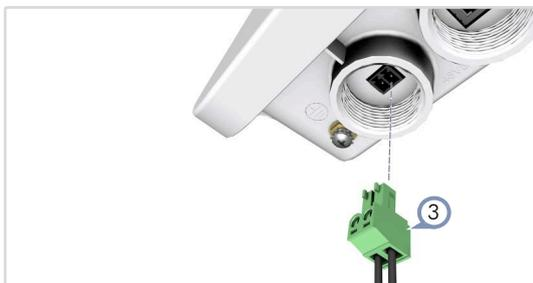
3. Wire the included DC terminal plug to a 48 VDC, 0.5 A source to provide power to the device. Follow the wiring scheme shown on the panel with the negative pole (-) on the left and the positive pole (+) on the right.
