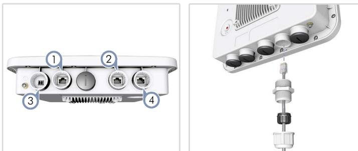
**i Note:** Port covers and cable glands should be tightened to a torque of 10 kgf.cm.
