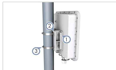
1. Use the included M6 screws to attach the mounting bracket to the device.
