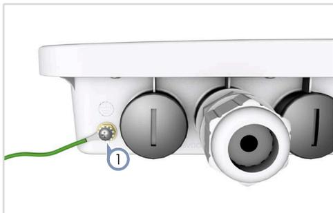
1. Ground the device by connecting a ground wire to the grounding point on the device and to nearby good earth.
