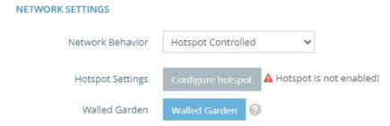
Support hotspot controlled in the network settings of wireless radio 5/2.4 GHz page.
