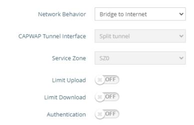
Support split tunnel in the network settings of wireless radio 5/2.4 GHz page.
