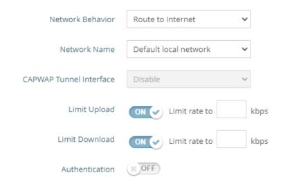
Support limit upload / limit download in the network settings of wireless radio 5/2.4 GHz page.
