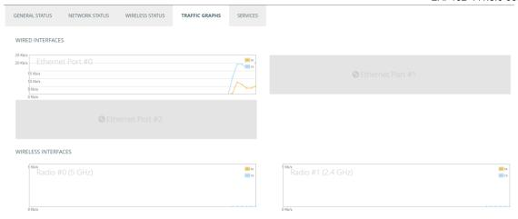
The Traffic Graphs section shows the data rate for the Ethernet ports and wireless interfaces.
