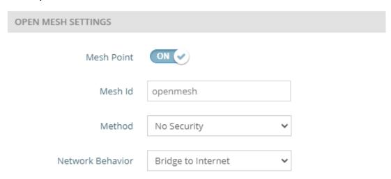
Support network behavior of Open Mesh feature in the Radio 5/2.4 GHz of Wireless page.
