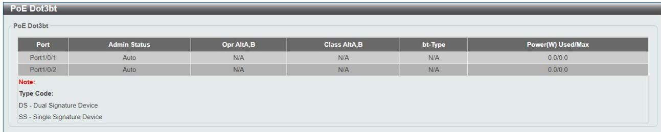
The screenshot shows a web interface for PoE Dot3bt configuration. It features a table with columns for Port, Admin Status, Opr AltA,B, Class AltA,B, bt-Type, and Power(W) Used/Max. Below the table is a 'Note' section with 'Type Code' definitions for DS (Dual Signature Device) and SS (Single Signature Device).
